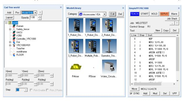
If any panel window is not appearing onscreen any longer then the best method to remedy the issue is to delete the \*.xml file in the simulation folder:
